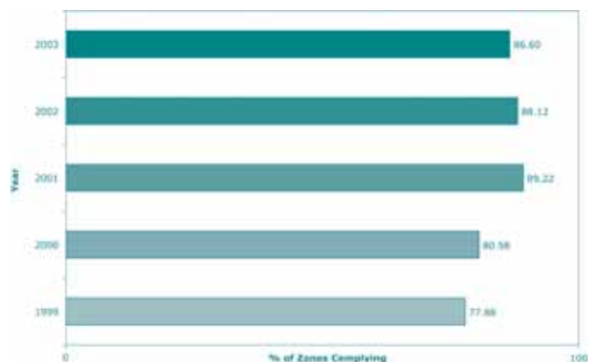
Figure 22: Water Supply Zones Complying with Aluminium Standards
