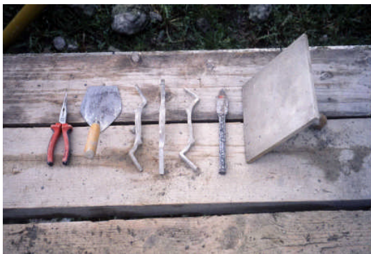
Examples of tools used in conservation works to scheduled masonry monuments.
