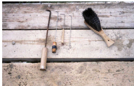
Examples of tools used in conservation works to scheduled masonry monuments.
