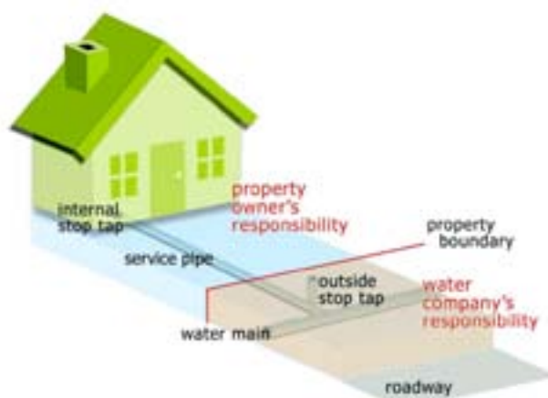
Figure 5.6 Typical Water Supply Arrangements
