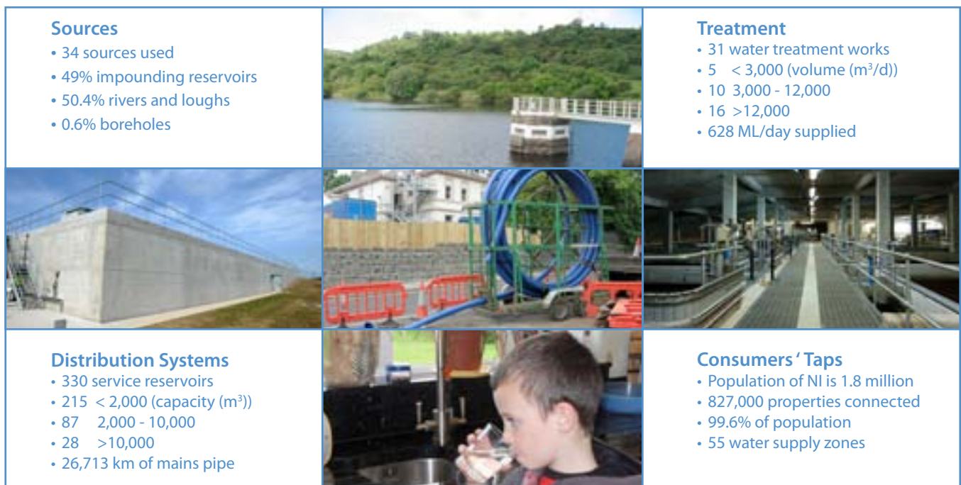
Figure 1.1: NI Water Supply Details
